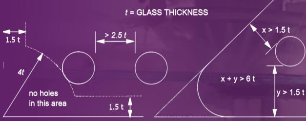
IF HOLES ENCROACH INTO THE EDGE OR CORNER ZONE, CHECK WITH MANAGEMENT OR OFFICE BEFORE TOUGHENING
